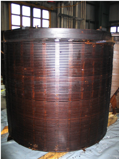
Fig. 11: Undamaged HV winding
